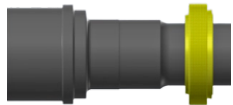
Location of the outer wheel bearing when used in a wheel hub for METRIC diff cover bolts
